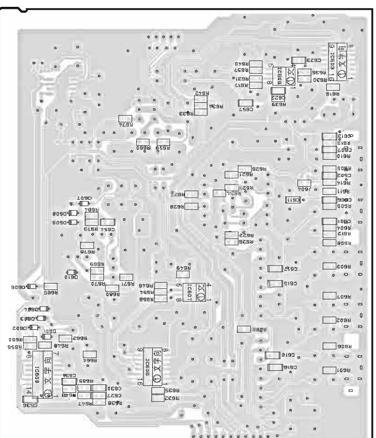
SUBTRANS (3) P.C.B. (Side B) Lead Free Solder Used
